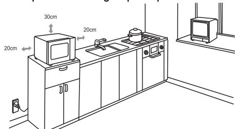
A minimum clearance of 7.9 inches (20cm) is required between the oven and any adjacent walls.
